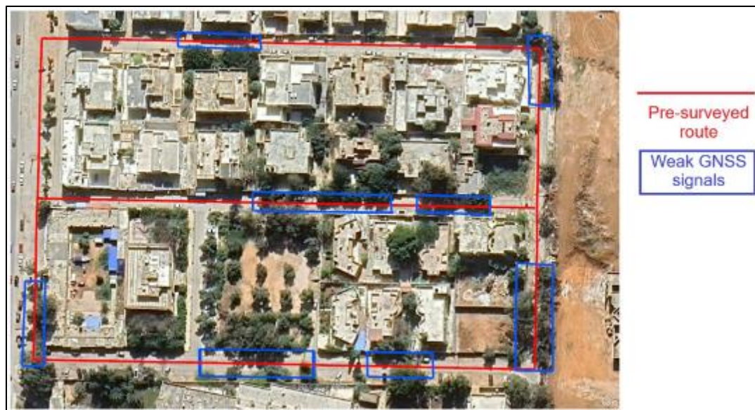
Figure 2 Testing pre-surveyed route with weak GNSS signal zones
