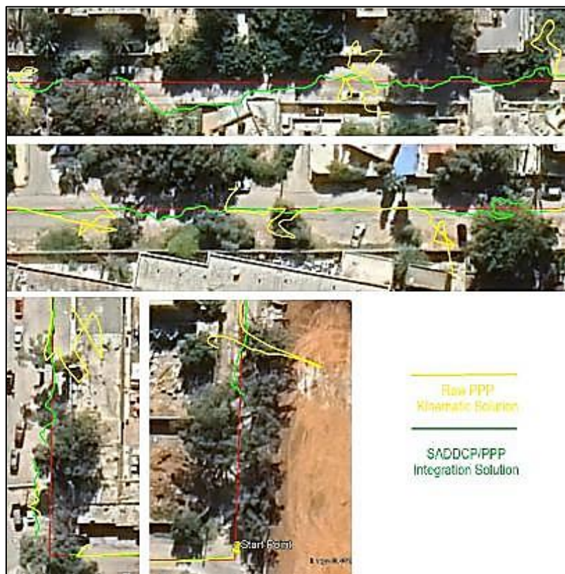
Figure 6 Raw kinematic PPP Vs. SADDCP/PPP integration in heavily obscured sky areas
