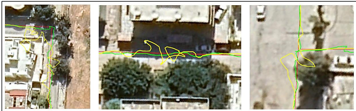
Figure 5 Raw kinematic PPP Vs. SADDCP/PPP integration in partially obscured sky
