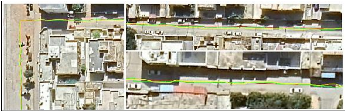
Figure 4 Raw kinematic PPP Vs. SADDCP/PPP integration in open-sky areas
