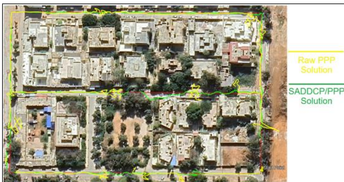
Figure 3 Raw kinematic PPP Vs. SADDCP/PPP integration in all testing area
